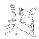
**2** - For use with Propane open the fuel compartment and insert a 1lb propane bottle and attach by pushing up and turning counter clockwise.
